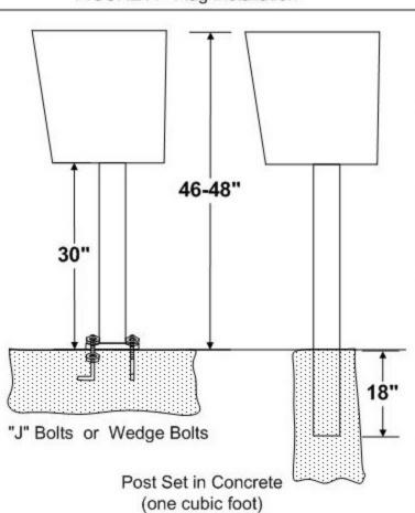
FIGURE C - Ground Installation
