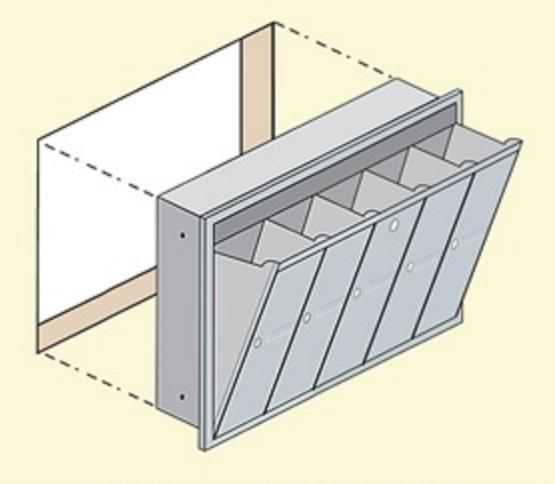
Recess mounted units fit into a rough opening and are secured with mounting hardware through the back or side panels.
