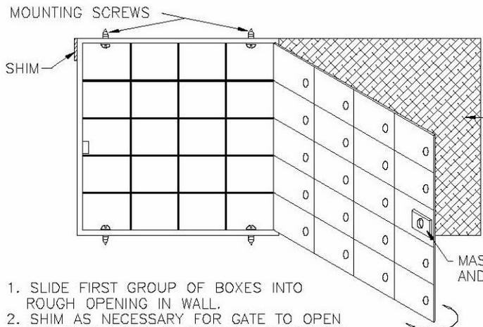
REFER TO ARCHITECTS CONSTRUCTION DRAWING FOR WALL DETAILS.
