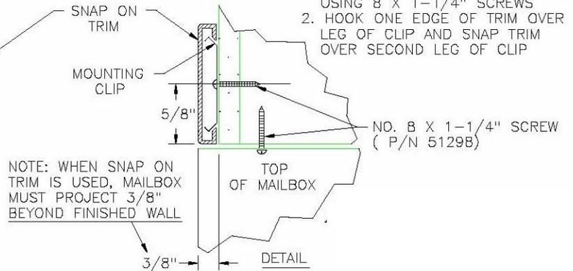
1. SCREW MOUNTING CLIP TO WALL USING 8 X 1-1/4" SCREWS
